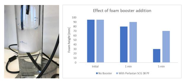
The test is performed in an in-house designed and build foam tester, based on circulating foam formation. The tests are performed in 1% solutions of the product in demineralized water.
