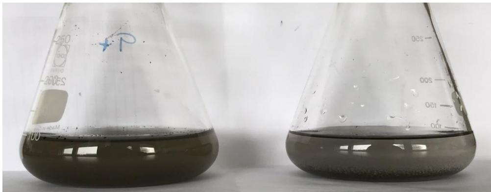
Dispersion of wood ash. 0.15% Ash. Left: Addition of 0.1% Polyaspartic acid Right: No addition. 1h after suspension.
