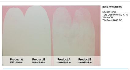
**Fig. 1** Black box cleaning test on a ceramic tile soiled with used cooking grease and aged for 5 hours at  $60^{\circ}$ C.
