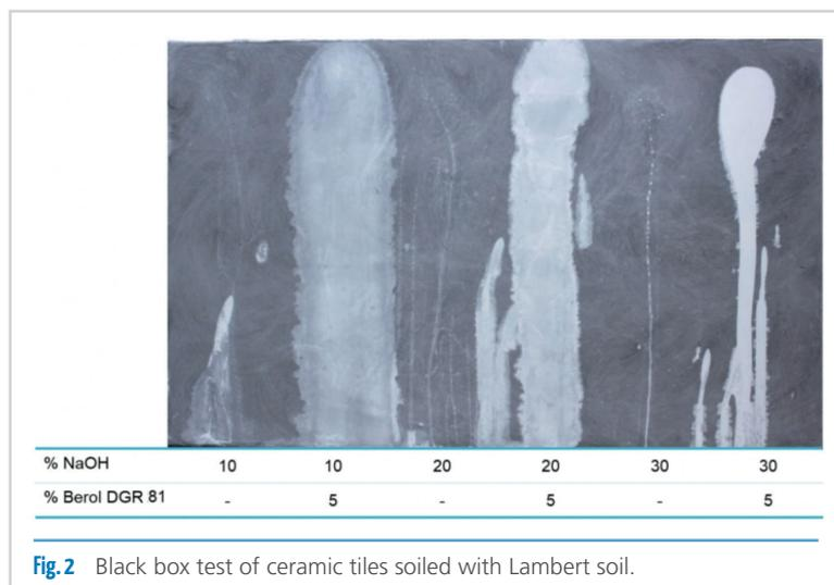
**Fig. 2** Black box test of ceramic tiles soiled with Lambert soil.
