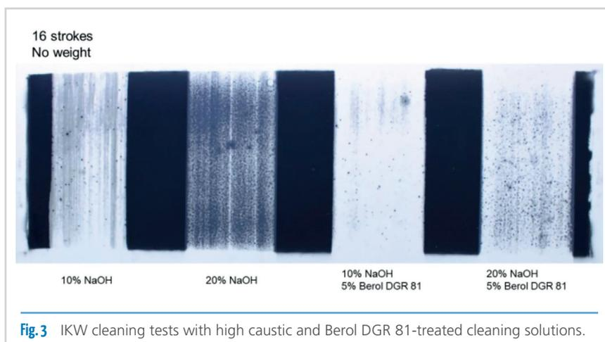
**Fig. 3** IKW cleaning tests with high caustic and Berol DGR 81-treated cleaning solutions.
