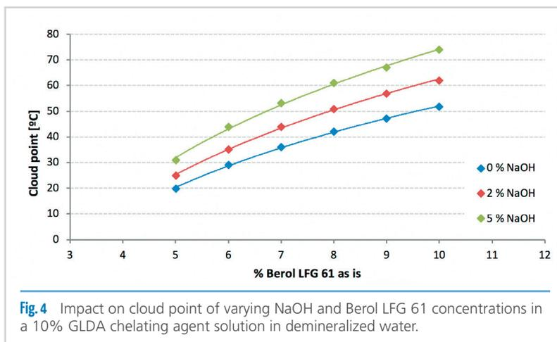
**Fig. 4** Impact on cloud point of varying NaOH and Berol LFG 61 concentrations in a 10% GLDA chelating agent solution in demineralized water.
